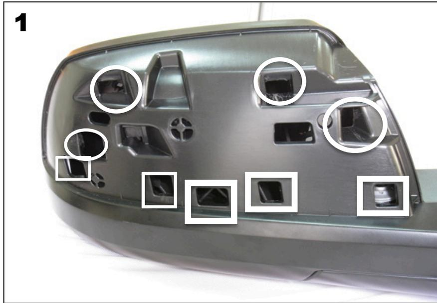
1. This picture shows 5 slots on the bottom in rectangles & 4 slots for clip insertion in circles.
